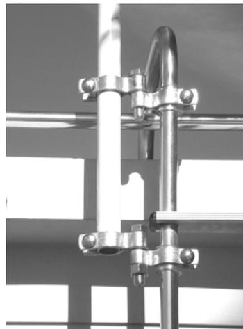
Once the brackets are in place, you can quickly put up the wind generator and mast (with wires already threaded through the mast and quick-disconnector extending out the bottom).
